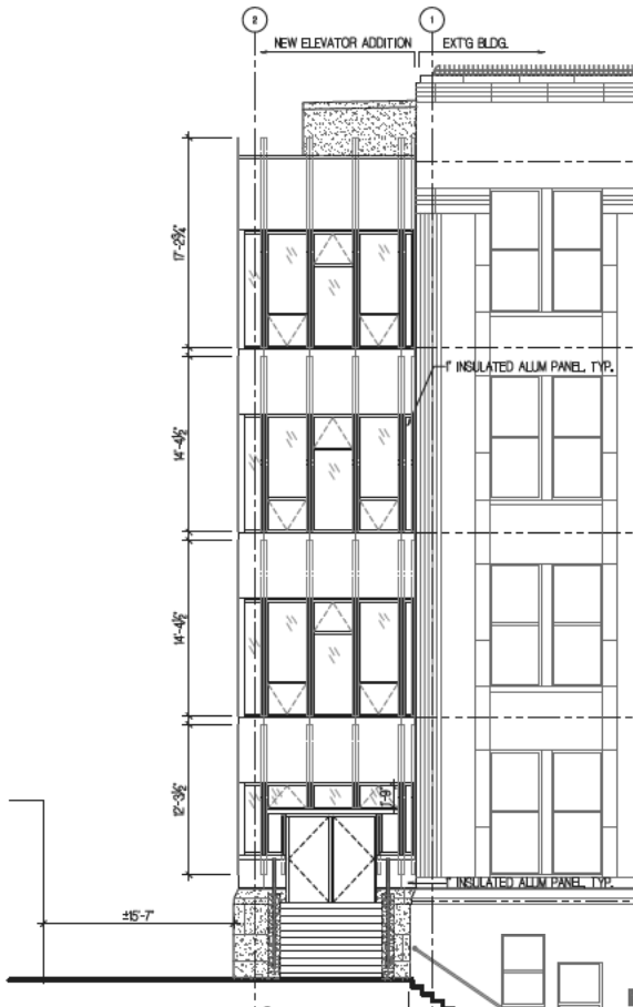
3.1 ELEVATOR ADDITION @ WEST FACADE (W/O PANELS)
